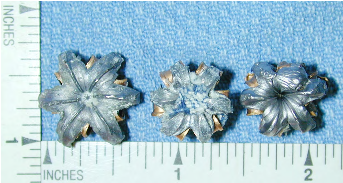
9 mm Federal 147 gr HST recovered from: BG - 4LD - Human Tissue (through Gore-Tex jacket, fleece vest, cotton shirt)
