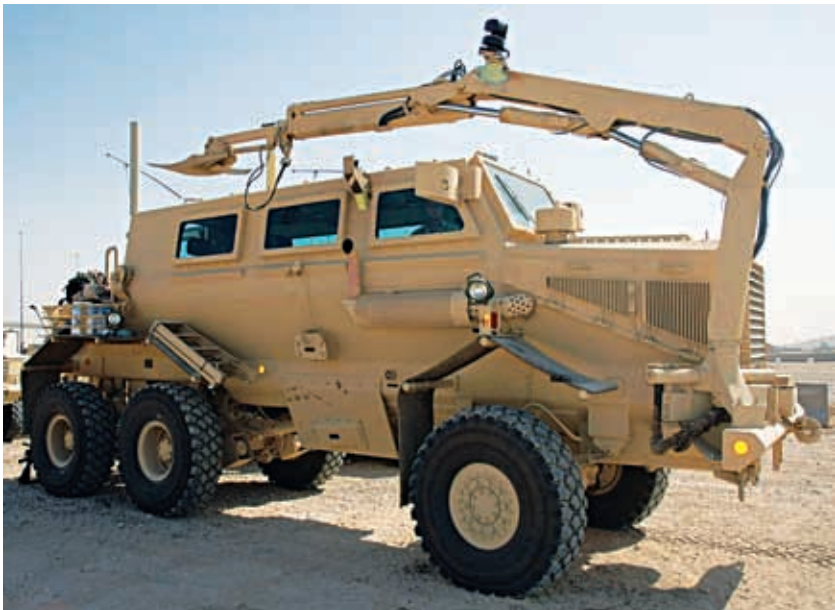
The Buffalo MPCV is designed to counter IEDs by safely detecting and inspecting them. ( Department of Defense )
